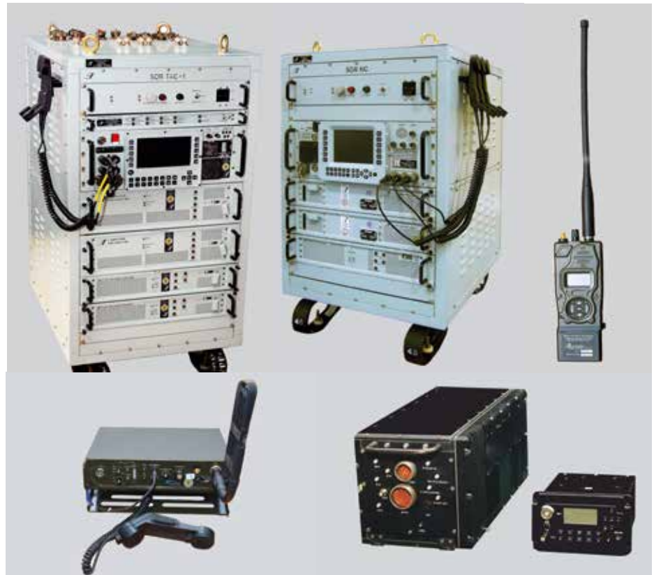
SDR form factors (clockwise from top left): SDR Tactical; SDR Naval Communication; SDR Hand-held; SDR Airborne and SDR Manpack
