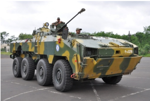
Wheeled Armoured Platform (WhAP) 8x8 & Add-on armour components
